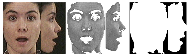
Fig. 2. Dual-view face image, HSV color-based segmentation for Face markers and segmented face and face-profile regions
