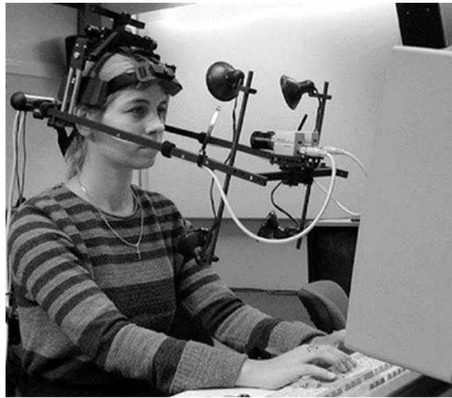
Fig. 9. Head-mounted two-camera device.
