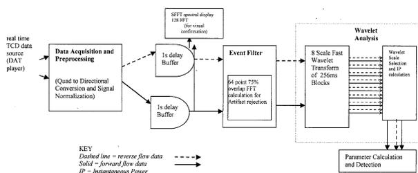
Fig. 1. A schematic diagram of the discrete wavelet transform (DWT-1) detection system.
