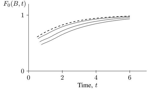
Figure 2. CDF of battery life,  $F_0(B, t)$  for different threshold values. The dashed line represents the case of no threshold, lines beneath are thresholds at  $V = 0.1$ ,  $V = 0.3$  and  $V = 0.5$ . Note the jump at the start. This is the probability that the initial non-charging period is long enough for the battery life to end with no charging periods having occurred. The parameters here are set to  $\lambda = 3$ ,  $\mu_h = 2$ ,  $\mu_\ell = 1$ ,  $B = 1$  and  $\alpha = \beta = 1$ .
