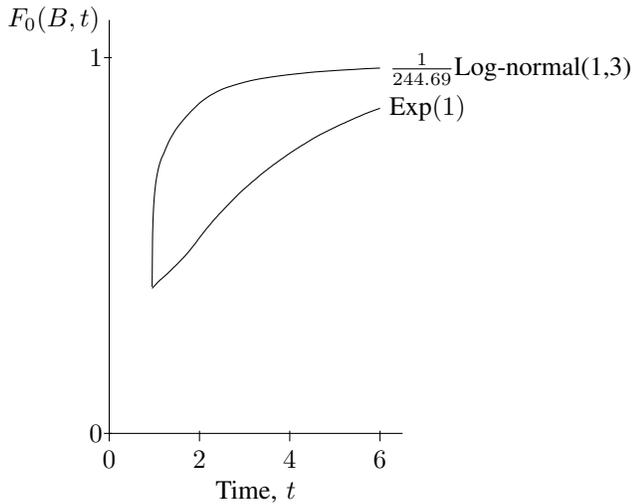
Figure 6. Simulated CDF showing the effect of changing the charging period distribution. All simulations run with  $B = 1$ ,  $\lambda = 3$ ,  $\mu_h = 2$ ,  $\mu_\ell = 1$ ,  $\beta = 1$  and  $V = 0.5$ . The charging period for the lower curve is exponentially distributed with parameter 1 as earlier in this paper. The charging period for the upper curve is a scaled log-normal distribution such that both on period distributions have mean 1.
