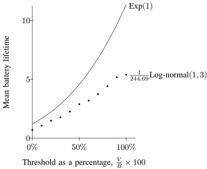
Figure 5. Mean battery life against threshold value  $V$  for different charging period distributions. Both on period distributions have mean 1. In the upper curve the distribution is exponential with parameter 1, in the lower points a log-normal distribution. The parameters here are set to  $\lambda = 3$ ,  $\mu_h = 2$ ,  $\mu_\ell = 0.5$ ,  $B = 1$ ,  $\beta = 1$  with charging period distribution either  $\text{Exp}(1)$  or  $\frac{1}{244.69}\text{Log-normal}(1, 3)$ .
