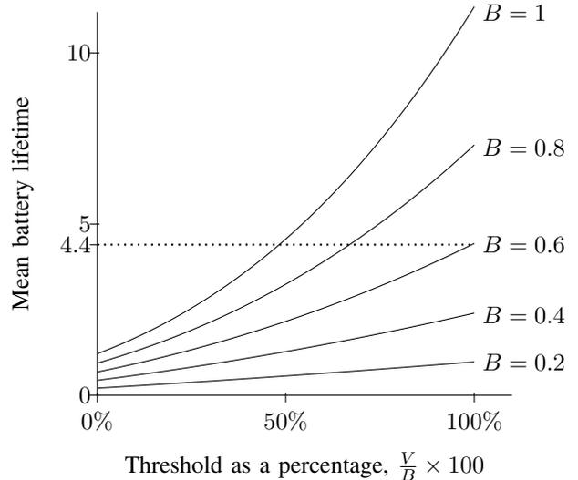
Figure 4. Mean battery life plotted against threshold value  $V$  for different battery capacities,  $B$ . We plot  $B = 0.2, 0.4, 0.6, 0.8, 1$  (from bottom to top). The dashed line shows how larger batteries with a low threshold can have the same mean battery life as smaller batteries with a higher threshold value. The parameters here are set to  $\lambda = 3$ ,  $\mu_h = 2$ ,  $\mu_\ell = 1$ ,  $B$  as labelled and  $\alpha = \beta = 1$ .
