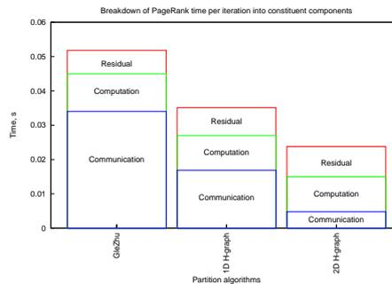
**Fig. 4.** Per-iteration execution time for 16-processor Stanford\_Berkeley PageRank computation.
