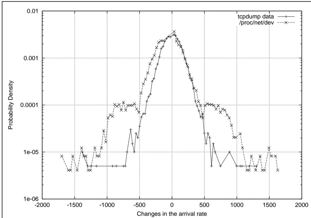
FIGURE 5. The plot displays the distribution of the changes in the packet event rate, measured over the same two-hour period using both `tcpdump` and `/proc/net/dev`.
