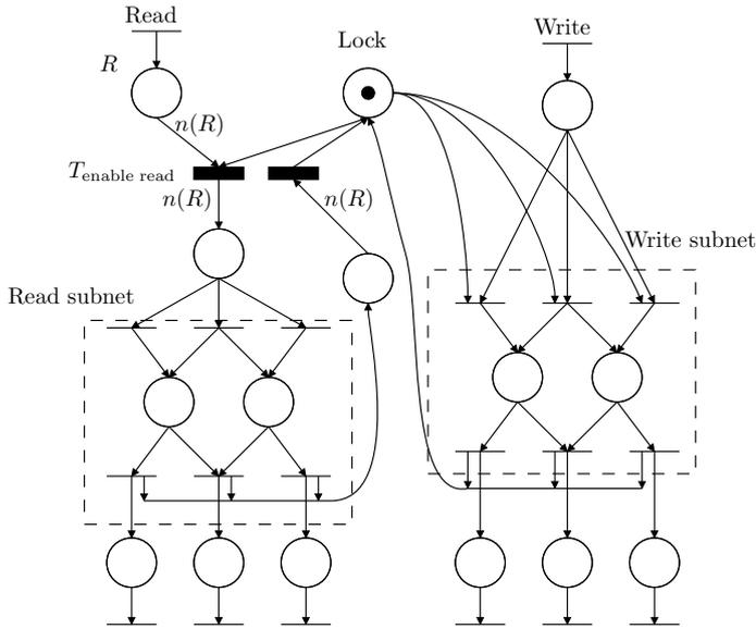
Fig. 1. SPN specifying concurrent access to a database. Solid transitions should be considered immediate transitions.  $n(R)$  denotes that the arc weight is the marking of place  $R$  just before the last firing of immediate transition  $T_{\text{enable read}}$ .
