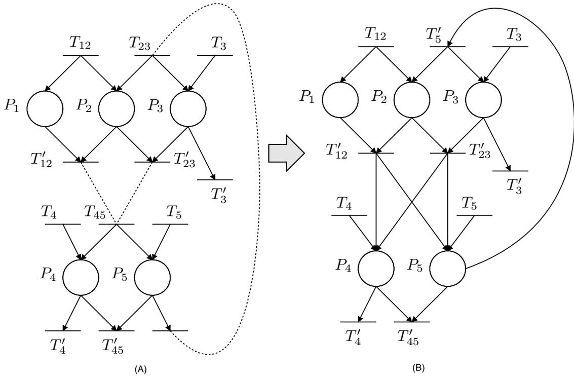
Fig. 6. Net considered in Example 2 of composition of BBs. (A) BBs to be composed. (B) Resulting net.
