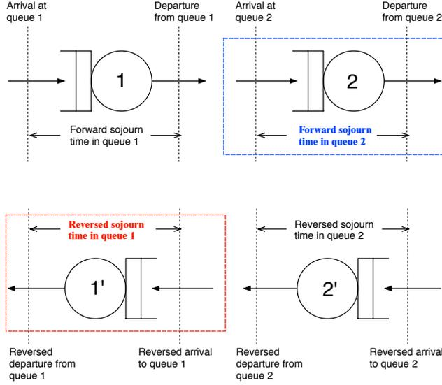
Figure 6: Two M/M/1 queues in tandem and the reversed process
