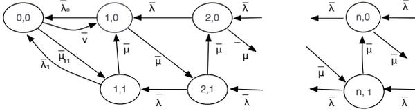
**Figure 9: Transition diagram of the reversed queue with Erlang-2 service**
