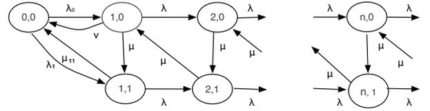
**Figure 2: Transition diagram of the queue with Erlang-2 service**
