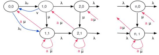
**Figure 3: Transition diagram for the Erlang-2 queue in isolation**
