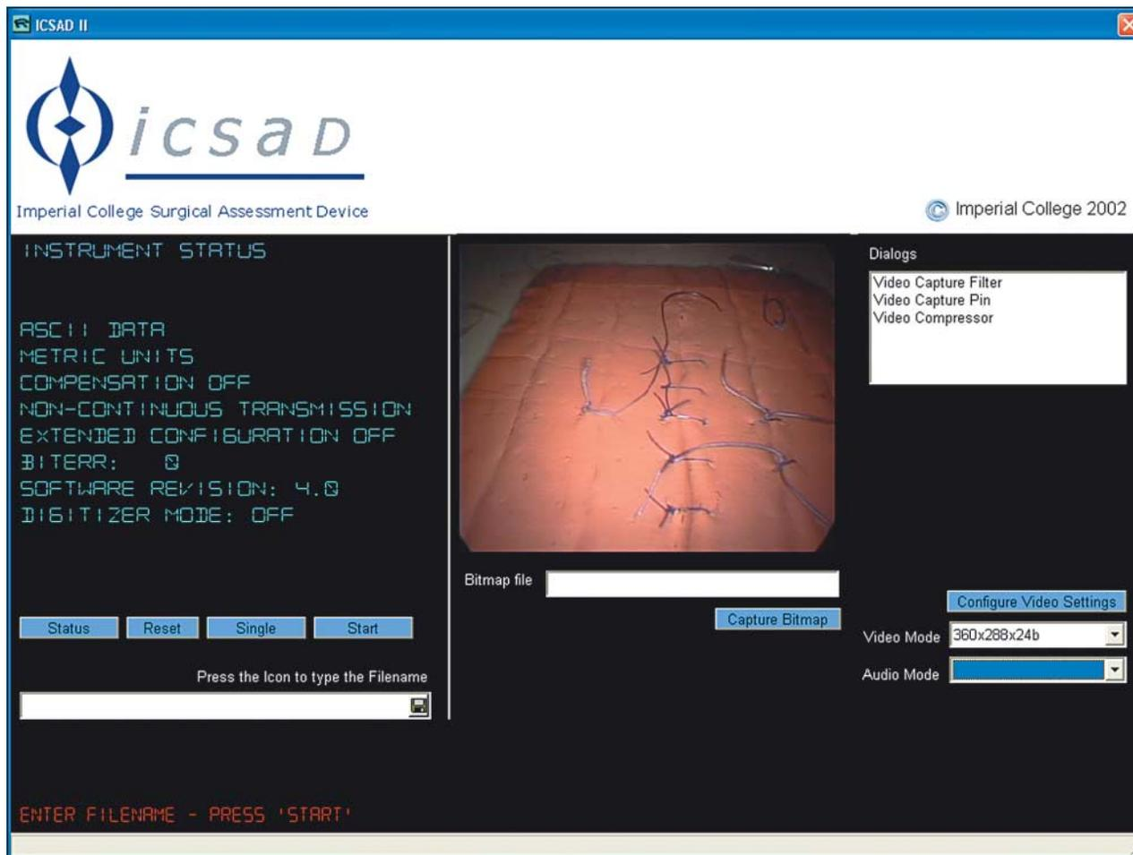
**Figure 2.** Imperial College Surgical Assessment Device (ICSAD) data and video acquisition component. On the left side information regarding the commercially available electromagnetic tracking system (Isotrak II; Polhemus Inc, Colchester, Vt) is displayed along with the tracking status. On the right the video capturing window displays the endoscopic surgical scene. Both motion and video streams are recorded using the same time stamp succeeding in perfect synchronization.
