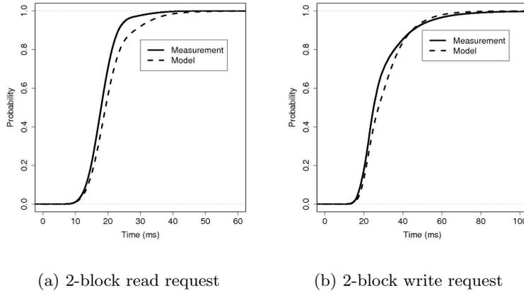
**Fig. 3.** Cumulative distribution functions of RAID 0-1 I/O request time on a 4 disk RAID system ( $\lambda = 0.02$  requests/ms)
